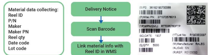
Figure 3: Material information binding to Reel ID
