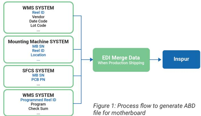
Figure 1: Process flow to generate ABD file for motherboard
