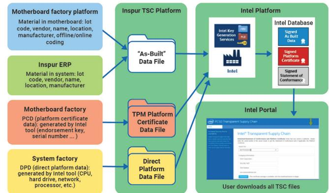
Figure 4: System factory TSC file upload & customer download process
